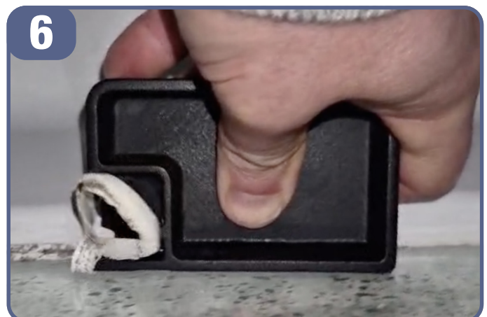
The SafestCut can be used in the opposite direction if required for a cleaner sealant removal
