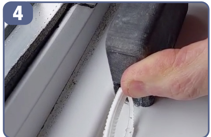
The SafestCut can be used flat or upright, which is useful when removing sealant from behind taps
