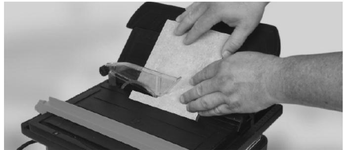
Switch on the machine and feed the tile through the cutting blade. When the cut is complete, switch off the machine.
