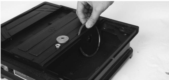
Position the blade against the blade carrier with the directional arrows on the blade facing anti-clockwise. Replace the blade washer and blade securing nut. Then replace the splashboard and secure with screw.
