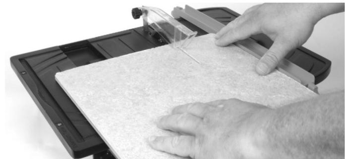
Maintaining an even pressure, hold the tile against the cutting guide and push steadily through the cutting wheel. When the cut is complete, switch off the machine.
