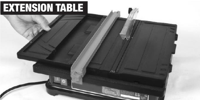
Slide out extension table, following arrow direction. After use, clean and remove any tile debris before retracting the extension table.
