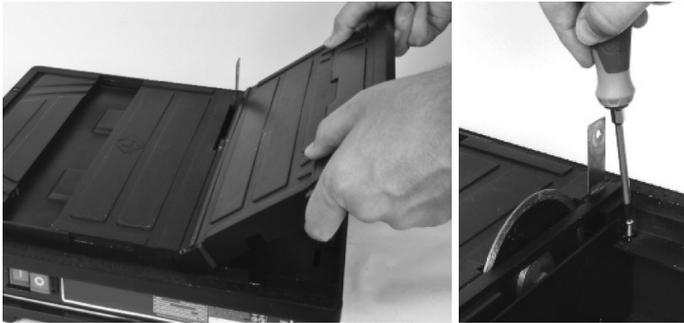
To fit or replace the cutting blade, first carefully lift the hinged section of the table top. Remove screw from splashboard and remove the splashboard to allow access. Remove blade securing nut and blade washer.
