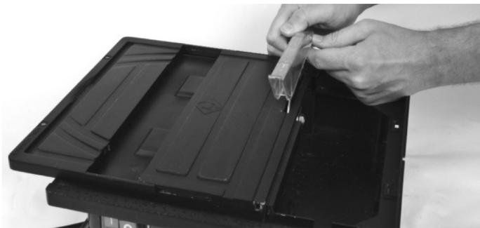
Close the table top hinged section and insert blade guard set behind the blade opening. Adjust the height accordingly.
