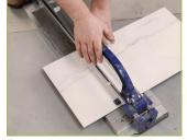
For repetitive straight cuts, it is worth investing in a Vitrex Manual Tile Cutter.
