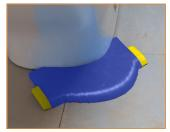
Use a Vitrex Profile Gauge to fit tiles around shaped areas such as pipes and wash basins.
