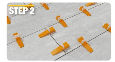
Position the tiles, aligning the sides and pushing them tightly against the clip. Slide a reusable wedge into each clip and tighten until tiles are snug against the bottom of the wedge.
