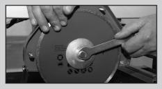
Whilst holding the shaft with the spanner wrench, turn the blade retaining nut clockwise to release using the hex wrench.
