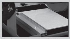
Place the tile in position on the cutting table so that it rests against the measuring scale and mitre guide.
