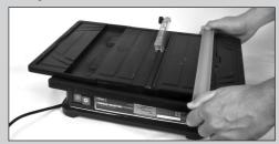
Place the Rip Guide on the table top and line up with the measurement graduations on either edge to the required size. When correctly aligned, tighten the rip guide securing nuts.
