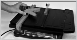
Press the Mitre Guide into place on the Rip Guide.
