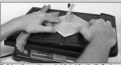
Switch on the machine and while holding the tile firmly in position, push the mitre guide steadily along the rip guide, feeding the tile through the cutting blade.
